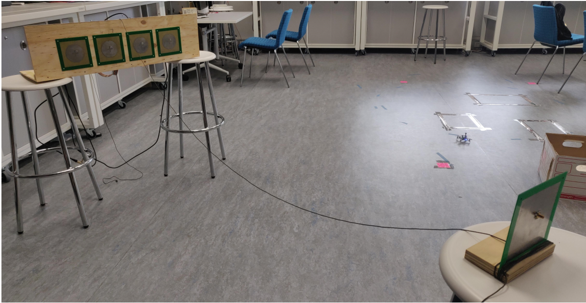
Figure 65: Photograph of phase-shift beamforming experiment, with array pictured in the upper left and the receiving element mounted in block in the lower right
